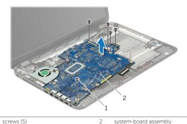
Turn the system-board assembly over.
